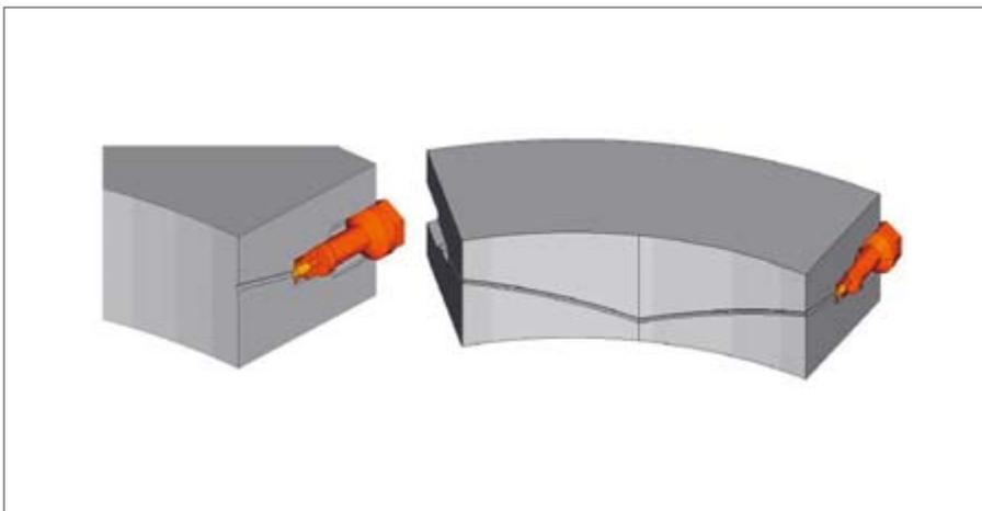
■ Fig. 8 – Pulse Feed principle with and without “zig-zag” distribution groove.
