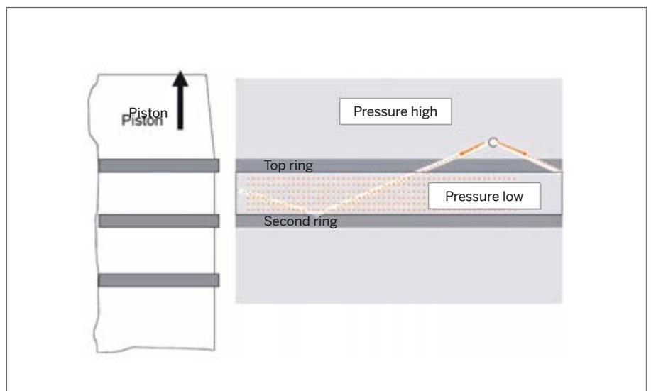
■ Fig. 9 – Function of the “zig-zag” distribution groove.
