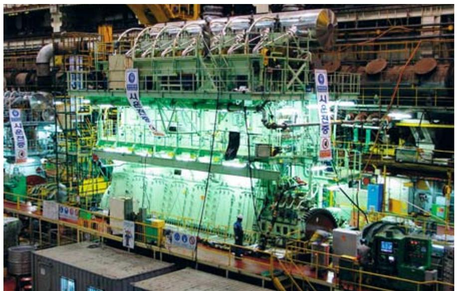
■ Fig. 2 – Wärtsilä 7RT-flex82C on test bed.
