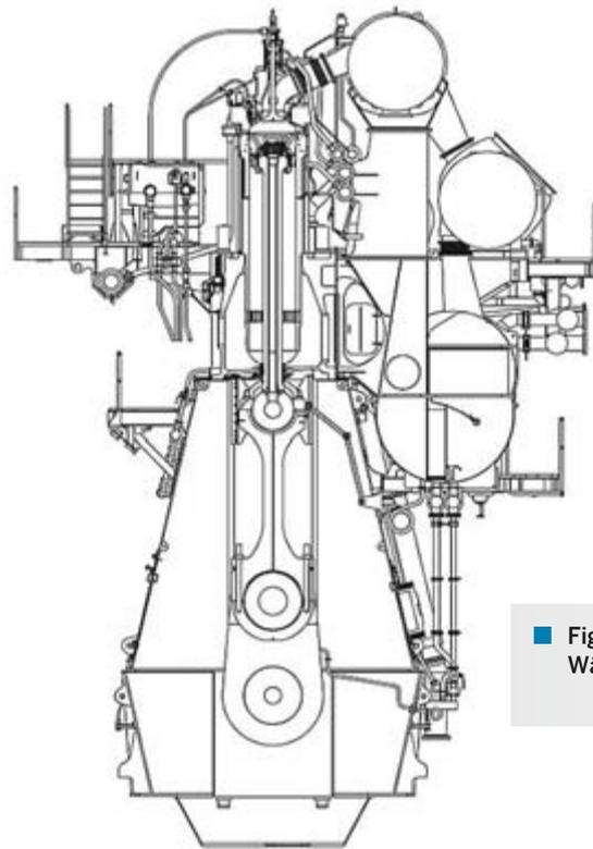
■ Fig. 1 – Cross section of Wärtsilä RT-flex82C.
