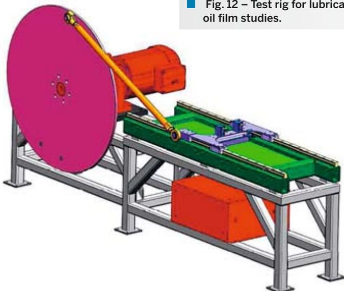
■ Fig. 12 – Test rig for lubricating oil film studies.
