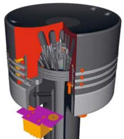
■ Fig. 13 – Instrumented piston for Wärtsilä RTX4 .
